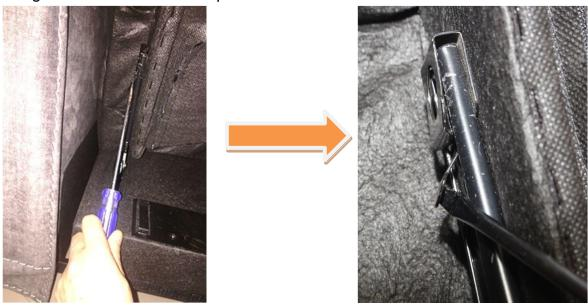
**3.** While holding the clip in the release position with the screwdriver, lift the corresponding side of the back cushion:
